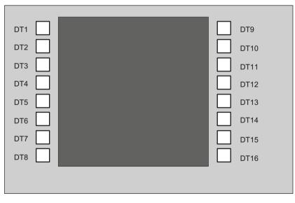
Image 1-7 Assignment of the direct keys to the vertical softkeys of an operator panel front
