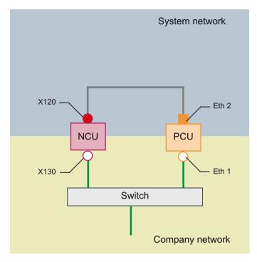
The NCU and PCU are connected via a crossed Ethernet cable.
