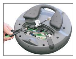
**2.** Insert the connecting cable in the appropriate entry (left or right).
