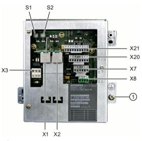
① Grounding screw M5 for potential equalization connection
