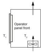
Heat dissipation using open-circuit ventilation
