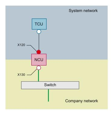
The TCU is connected to the NCU (directly) using a **crossed** Ethernet cable. On X130, the NCU is connected to a switch to the company network with a straight cable.
