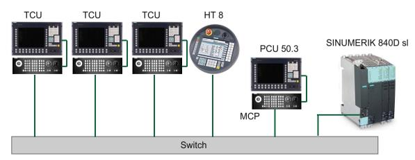
The mobile SINUMERIK HT 8 handheld terminal works on the thin client principle and combines the functions of an operator panel with a machine control panel.
