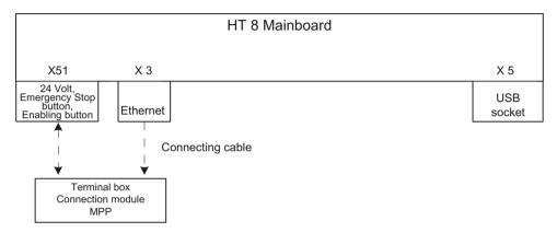
Image 4-1 Block diagram of HT 8 interfaces
