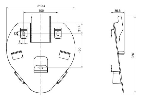
Image 10-2 HT 8 wall holder - dimension drawing
