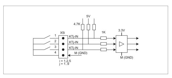
Image 1-5 Main circuit diagram of the input circuit for X51, X52 and X55
