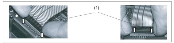
(1) Clamping frame of socket
