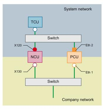
In this configuration, a switch is also required for the system network. All components are connected using straight Ethernet cables.
