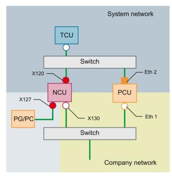
For service purposes a programming device is connected to the NCU at X127 as a standard DHCP client (automatically obtain an IP address). An NCU is a standard DHCP server on X127. On X127, the NCU occupies the fixed IP address 192.168.215.1 with the subnet mask 255.255.255.224.
