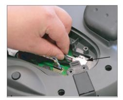
**4.** Connect the RJ-45 connector to the Ethernet socket.
