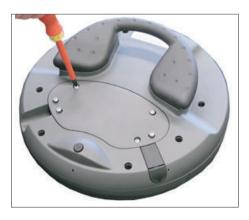
Open the cover by unscrewing the six PT screws (4 x 20 mm) approximately 1 cm. To do this, use a Phillips size 2 screwdriver. 5.4 Connecting cable
