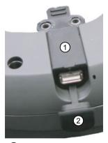
① Connector with integrated USB connection
