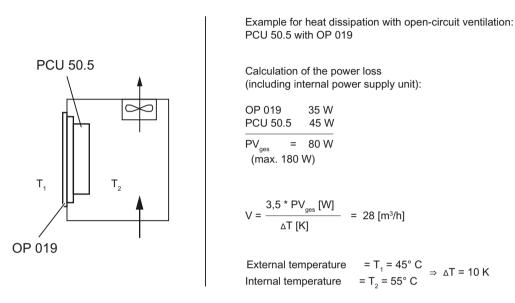
Image 1-2 Calculating heat dissipation for PCU 50.5 with OP 019
