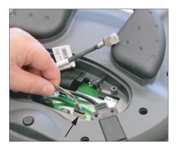
**3.** Press the plug connector firmly into the power supply socket.
