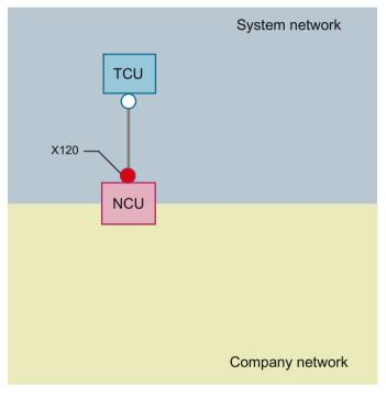
A direct Ethernet connection is used to connect a TCU to X120 of the NCU. NCU and TCU are suitably preconfigured with IP addresses.
