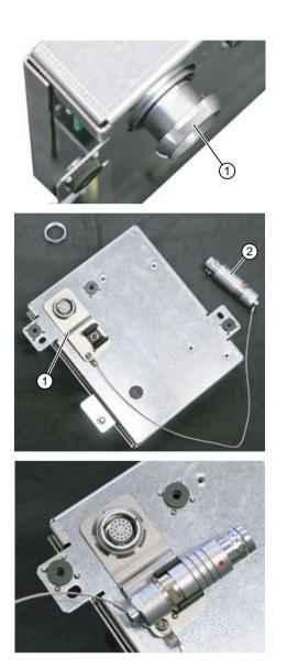
**1.**Unscrew the fixing nut ①.
